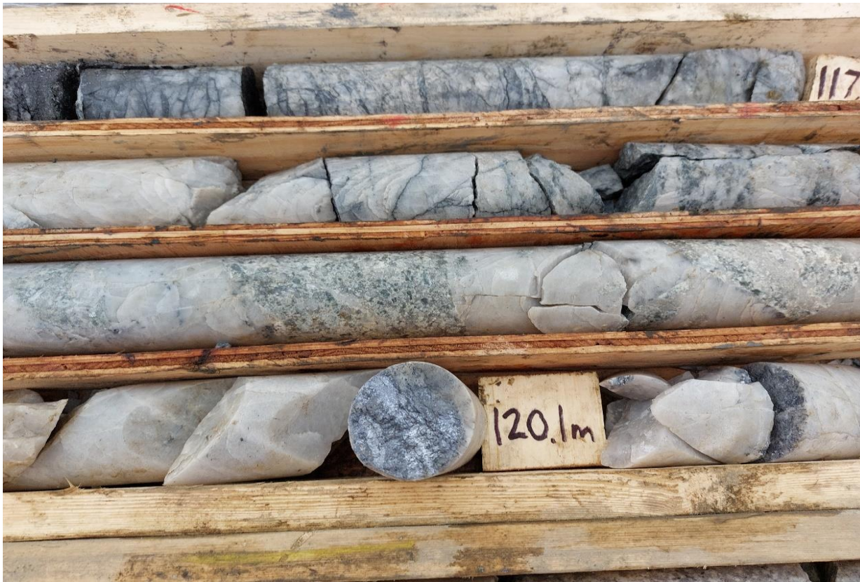
Figure 1: Representative photo of molybdenum mineralization identified near the end of drill hole NL-22-74
